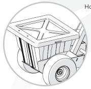
Hopper holds between **35 - 40 pounds** of dry line marking material.
