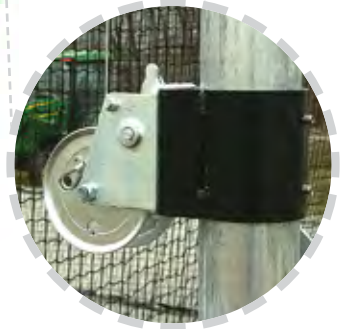
TENSIONING END Three pole mounted winches.
